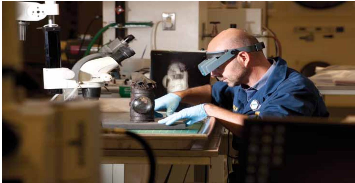
Tending the light: Chief conservator Paul Mardikian examines the Hunley's lantern, a whale-oil light used mainly for signaling. The lantern was highly degraded, with some parts missing. Mardikian used X-rays showing the lantern's "ghost" to reconstruct missing parts.
