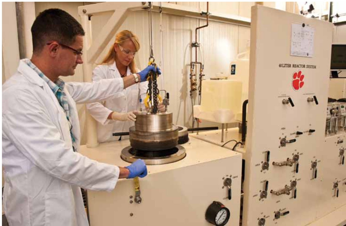
Nestor Gonzalez-Pereyra, a chemical engineer with the Lasch Center, and conservator Liisa Nasanen open the top of a canister where salt-impregnated metal artifacts undergo treatment in the center's patented subcritical reactor.
