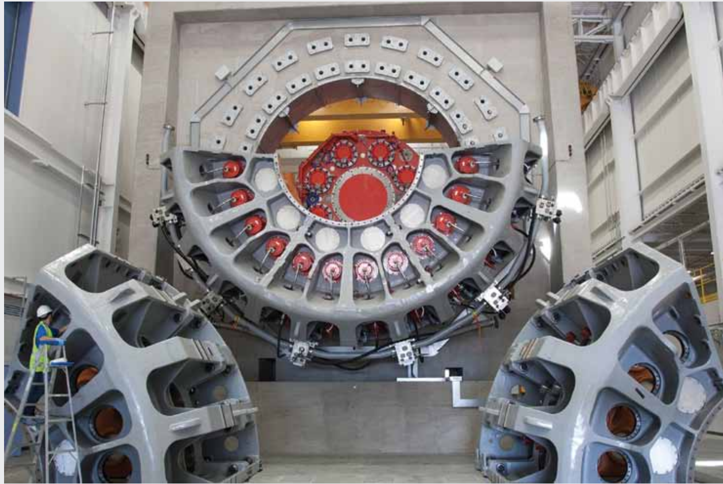
One of two test bays designed to put wind-turbine drivetrains through their paces. This one can handle equipment rated at up to 15 megawatts.
