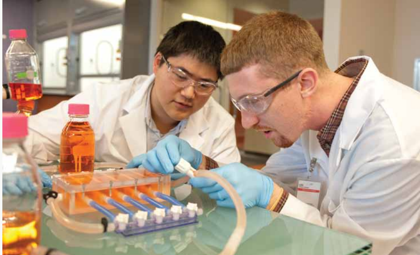
James Chow (left) and Lee Sierad (right) work on the vascular bioreactor for testing artery scaffolds, using the Patewood facility.
