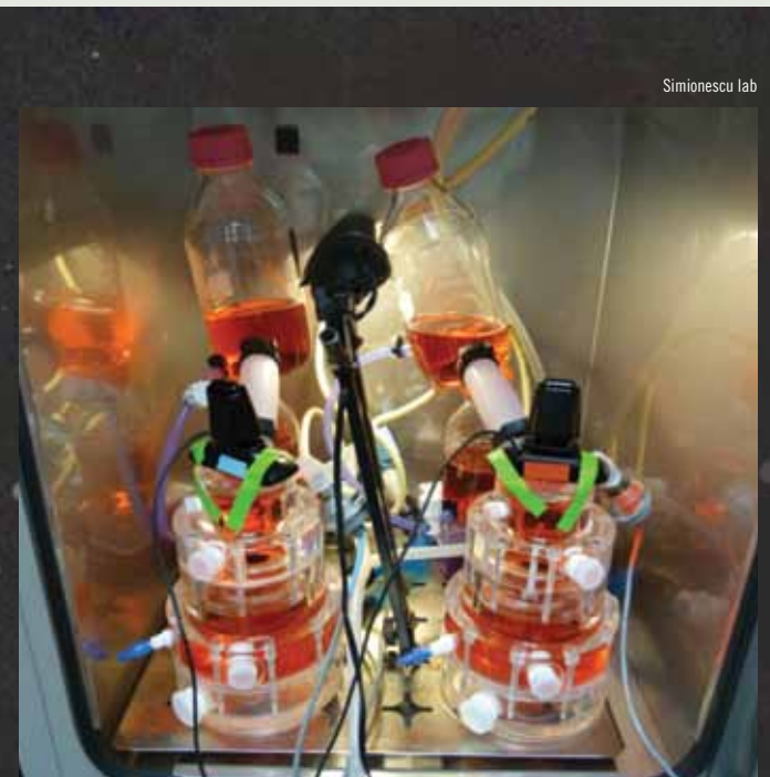
Above: Two heart-valve bioreactors, designed and built at Clemson, work in tandem. Below: A porcine aortic heart valve open and closed in the bioreactor.
