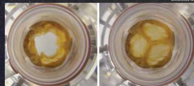
Above: Two heart-valve bioreactors, designed and built at Clemson, work in tandem. Below: A porcine aortic heart valve open and closed in the bioreactor.
