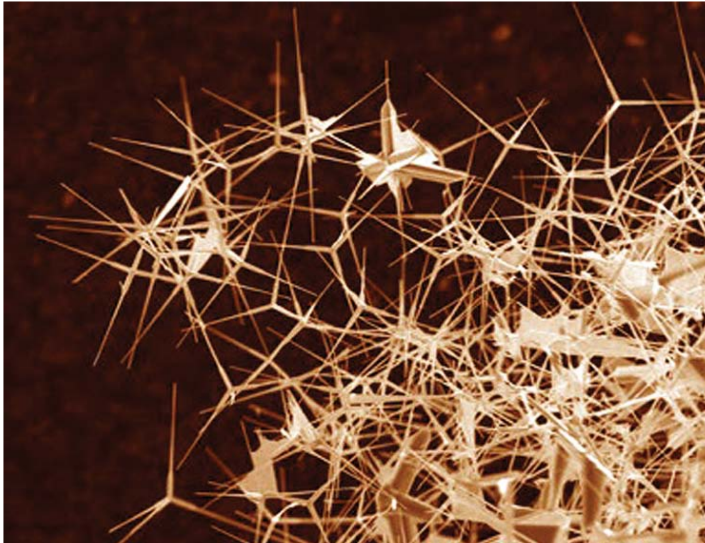
The Rao lab coated zinc oxide nanotetrapods with gold and created a biomolecular sensor.
