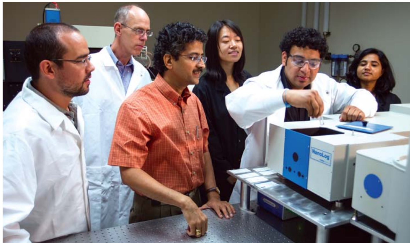
Apparao Rao (in orange) and members of his lab watch as Ramakrishna Podila (Rama) loads a cuvette with graphene quantum dots into a photoluminescence spectrometer. Others include (from left to right): Mehmet Karakaya, Herbert Behlow, Jingyi Zhu, and Deepika Saini. Rama and Rao's work on the origin of photoluminescence in graphene quantum dots is featured on the cover of the October issue of Advanced Functional Materials . The quantum dots "glow" under ultraviolet light and have great potential for biomedical imaging.
