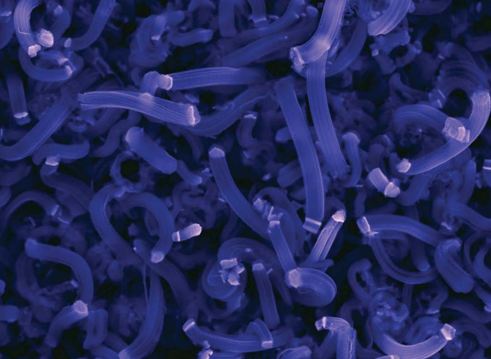
Helically coiled nanowires: This scanning electron microscopy image reveals a coveted helical shape synthesized in the Rao lab. The bright spot at the tip of each bundle indicates the catalyst particle. Image: Rao lab.
