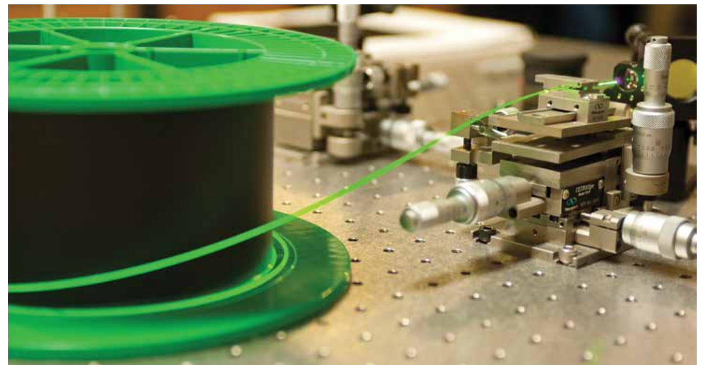
Research in Eric Johnson's lab develops the potential of lasers and optical fiber in manufacturing. This mid-infrared fiber laser shows green fluorescence under strong optical pumping.
