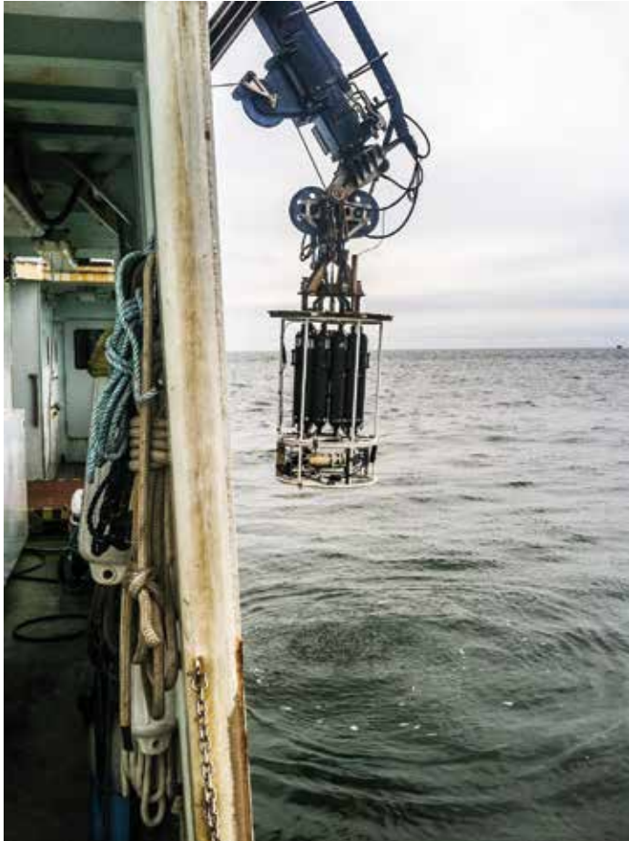
Above: An array of sampling equipment called a rosette is lowered into the Delaware Bay.
